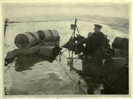
DROPPING DEPTH CHARGES ON SUBMARINES: "Stand by to release charge."
